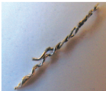
Fig. 3c Photograph of fractured segment revealing two separate instruments intertwined
