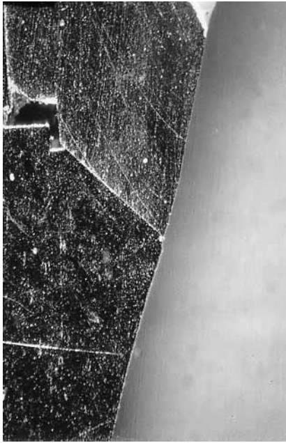
Fig. 5. Transverse section of a screw-retained specimen of an ITI implant. Compare the space between the implant and the crown with that seen in Fig. 4 in which the crown is cemented ( in vitro ) (original \times 40 ). Courtesy of Scott E. Keith.
